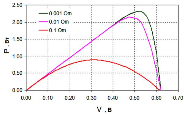
Fig. 5 – P-V characteristic of the SC at different values of  $R_{SH}$
