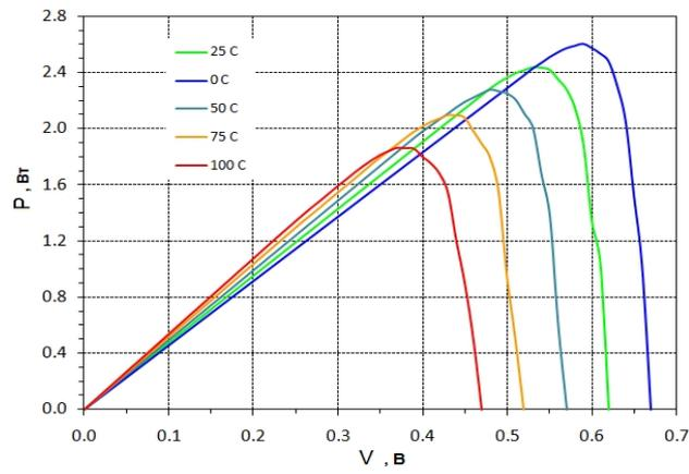
Fig. 9 – P-V characteristic of the SC at different values of the temperature
