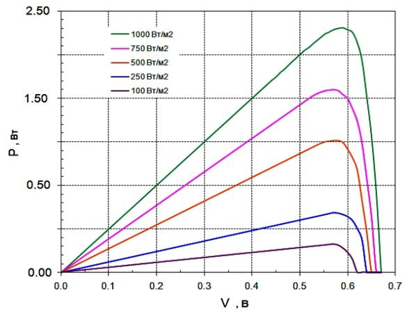
Fig. 11 – P-V characteristic of the SC at different lighting
