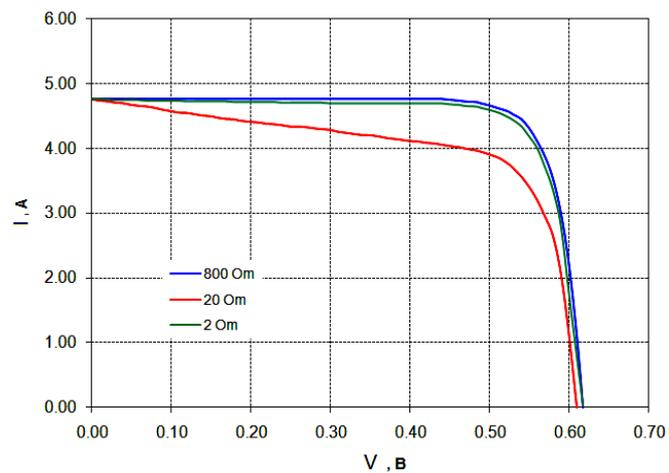
Fig. 6 – I-V characteristic of the SC at different values of  $R_S$
