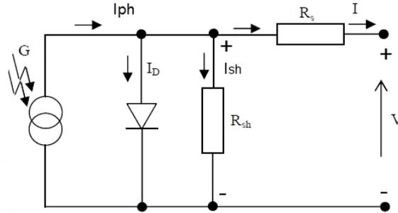
Fig. 2 – SC equivalent circuit by the single-diode model
