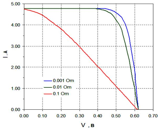
Fig. 4 – I-V characteristic of the SC at different values of  $R_{SH}$
