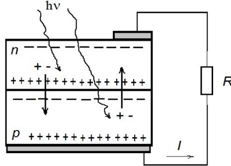
Fig. 1 – Solar cell structure
