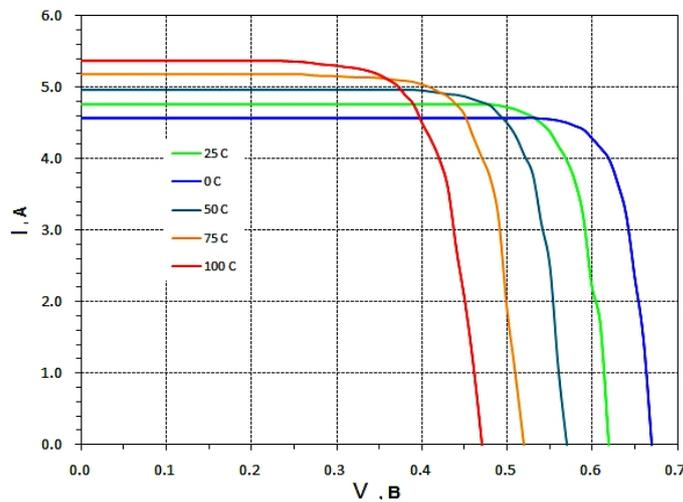
Fig. 8 – I-V characteristic of the SC at different values of the temperature
