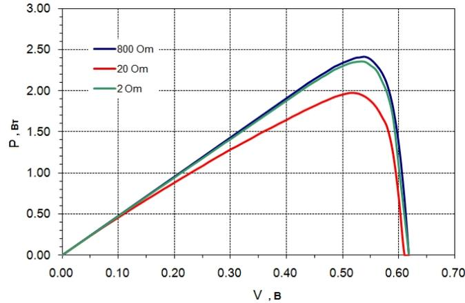
Fig. 7 – P-V characteristic of the SC at different values of  $R_S$
