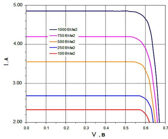
Fig. 10 – I-V characteristic of the SC at different lighting
