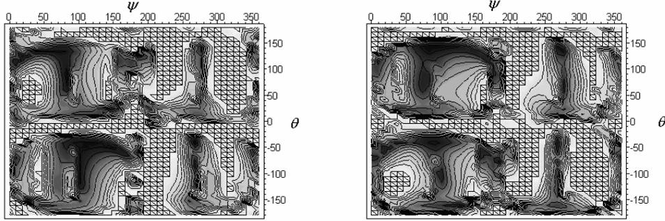
**Fig. 4** – Dependence of the reflection coefficients on the inclination angle of the anisotropy axis and the angle between the incidence plane and the plain containing anisotropy axis for twelve two-layer periods,  $d_2 = 100$  nm,  $d_1 = 40$  nm,  $f = 700$  THz: direct transmission (a); backward transmission (b)
