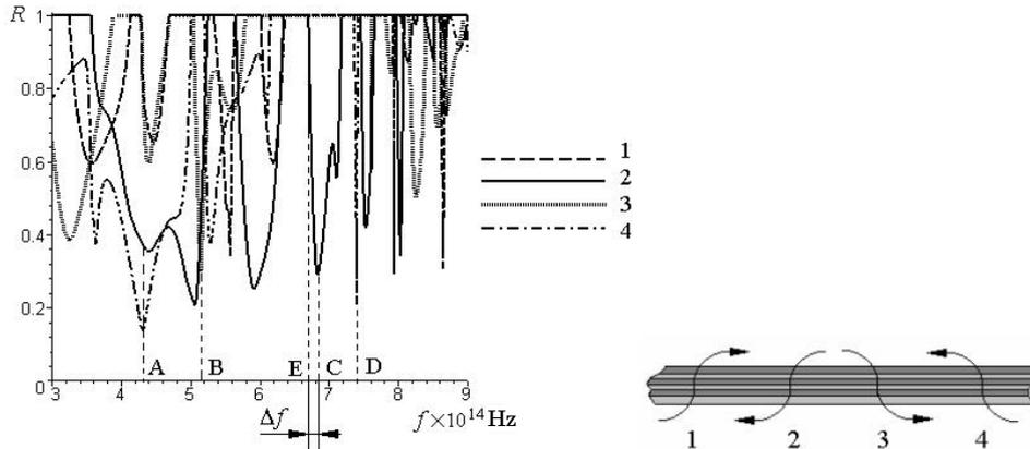
**Fig. 6** – Frequency dependence of the reflection coefficient at  $\theta = 21^\circ$ ,  $\psi = 169^\circ$
