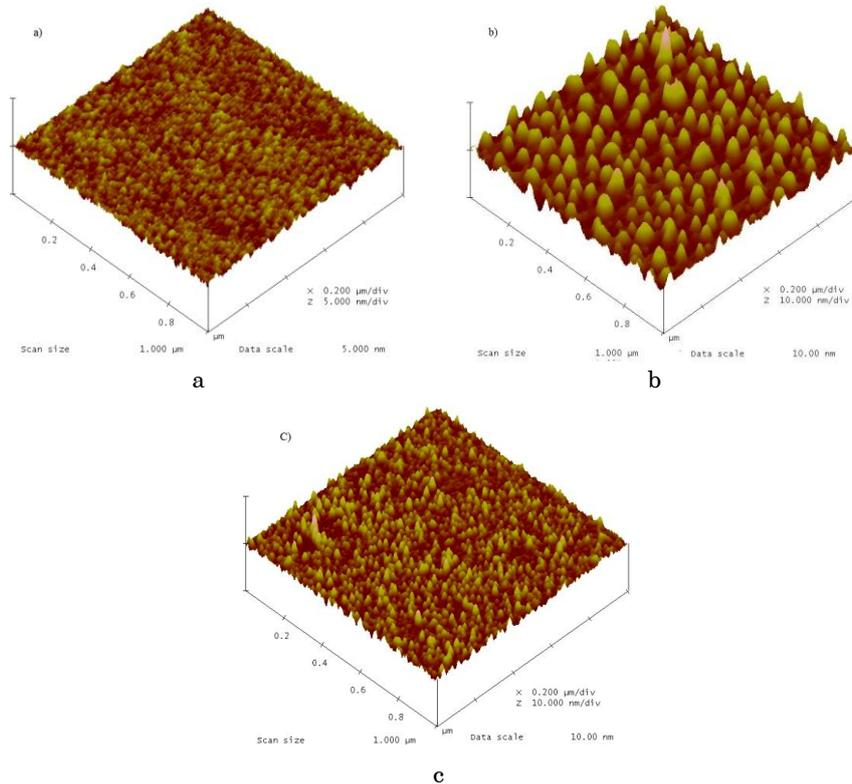
**Fig. 1** – AFM images of bare c-Si wafers a reference (a), the 2 min 3 % HF etched c-Si wafer (b), 10 sec intrinsic a-Si:H layer deposited on c-Si at  $T_{Fil} = 1500$  °C (c)
