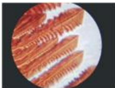
**Fig. 3** – Dendrite crystal growth features
