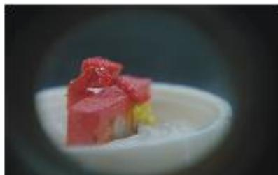
*Fig. 6 – Crystal with platinum electrodes*
