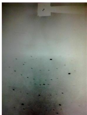
*Fig. 5 – X-Ray Laue Photograph (Transmission)*
