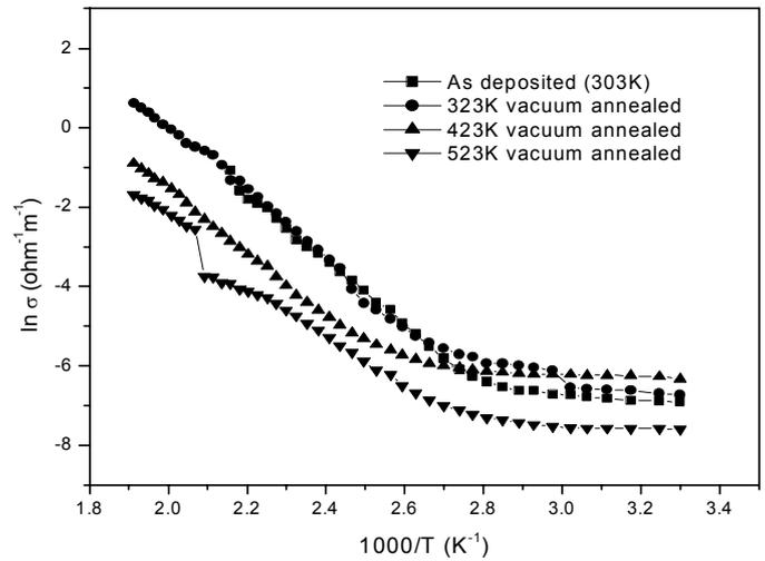
*Fig. 1 – lnσ Versus 1000/T for different ZTTBNc thin films*
