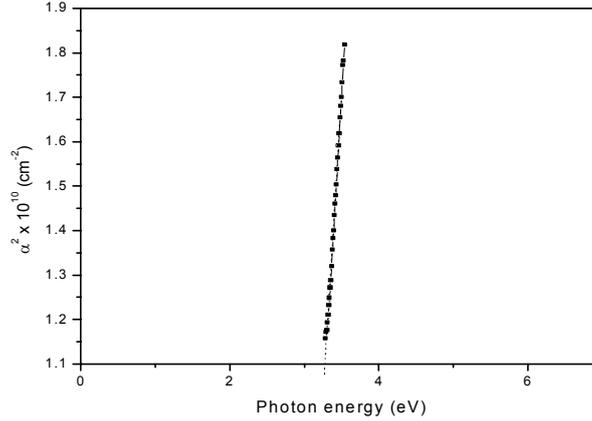
**Fig. 4** – Typical  $\alpha^2$  versus  $h\nu$  graph for as deposited ZTTBNc thin film
