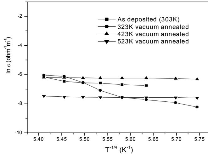
**Fig. 2** –  $\ln \sigma$  Versus  $T^{-1/4}$  for different ZTTBNc thin films
