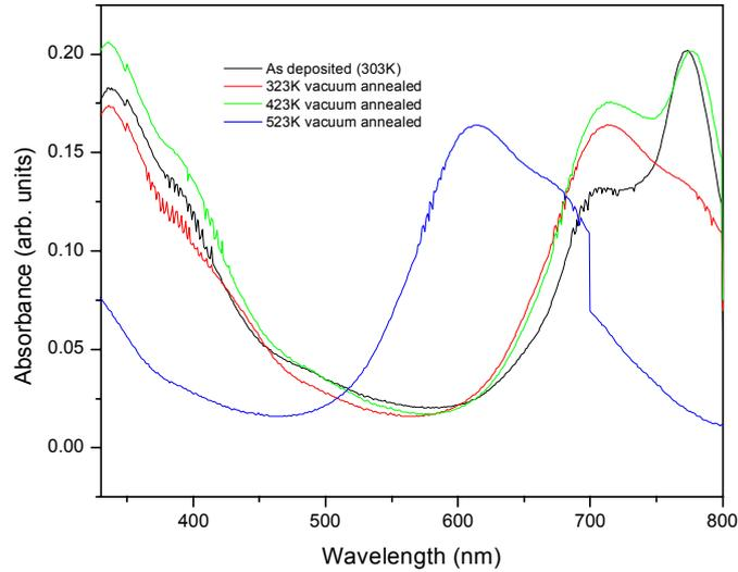
**Fig. 3** – Absorption spectrum of different ZTTBNc thin films
