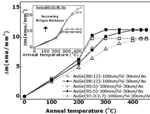
**Fig. 5** – Effective thickness of Ni layer transformed to non-magnetic phase on annealing at various temperatures. ( $\Delta m$  is the decrease in magnetization per unit area)
