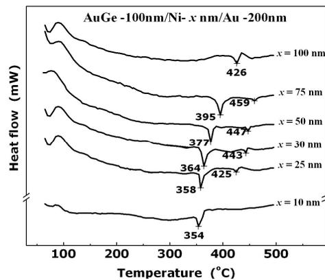
**Fig. 7** – DSC scans for samples with metallization structures with eutectic AuGe (88 : 12) alloy layer and different Ni layer thicknesses
