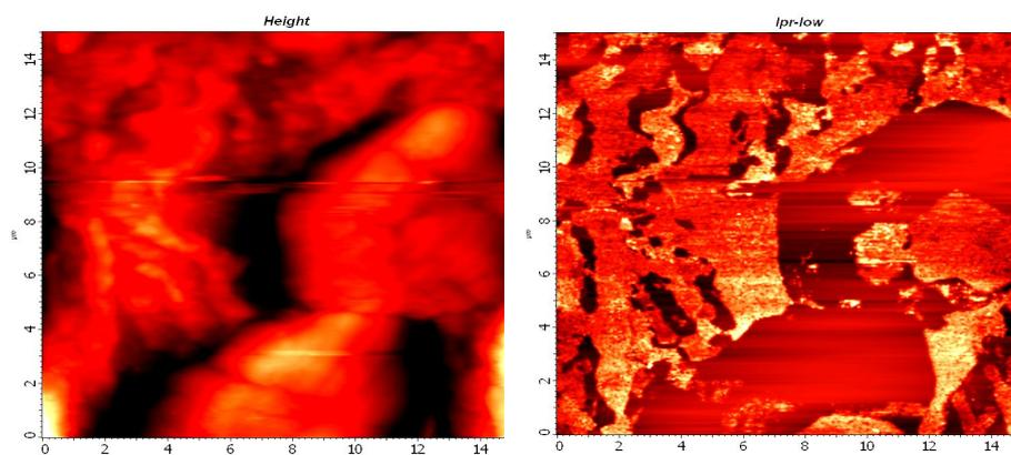
**Fig. 8** – Surface topography and current mapping of AuGe/Ni/Au which shows the least contact resistance
