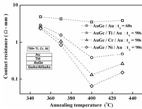
**Fig. 2** – Contact resistance as a function of anneal temperature for AuGe/TM/Au. TM = Ti, Cr and Ni or none. The lines are a guide to the eye
