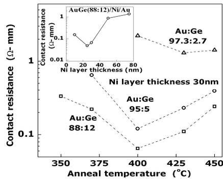
**Fig. 3** – Contact resistance Vs anneal temperature for different AuGe compositions and Ni layer thicknesses
