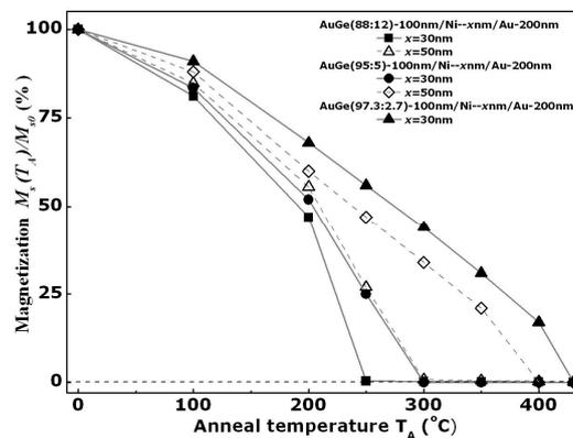
**Fig. 4** – Decrease in magnetization upon annealing, for contact metallization structures with three AuGe alloy compositions and different Ni layer thicknesses
