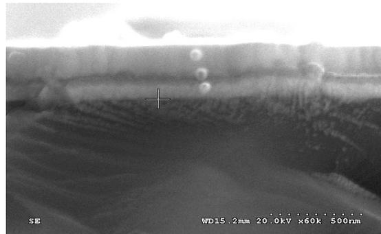
**Fig. 6** – Cross sectional SEM of AuGe (88 : 12 wt %) - 100 nm / Ni - 25 nm / Au - 200 nm annealed at 300 °C and cooled down to room temperature
