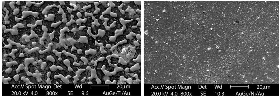
**Fig. 1** – SEM micrographs of the surface of AuGe/Ti/Au and AuGe/Ni/Au contact metallization structures, annealed at 400 °C
