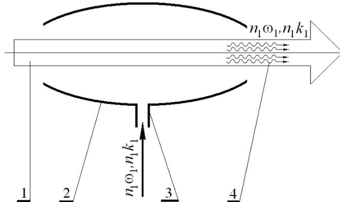
**Fig. 13** – Structural design of the optical (quasi-optical) modulator of the electron beam. Here: 1 – nonmodulated input signal; 2 – barrel-shaped multiharmonic optical (or quasi-optical) resonator; 3 – the resonator 2 input for a cluster electromagnetic signal with the frequency spectrum  $n_1\omega_1, n_1k_1$ ; 4 – modulated electron beam at the system output, i.e., the excited cluster SCW with the same (as signal) frequency spectrum  $n_1\omega_1, n_1k_1$
