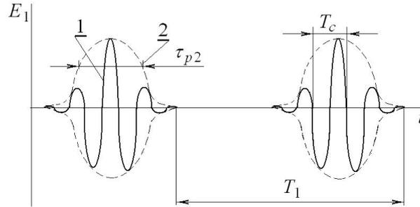
**Fig. 1** – Illustration of the conception of femtosecond electromagnetic pulse (radio-pulse). Here: 1 – instantaneous electric field intensity of radio-pulse; 2 – radio-pulse envelope;  $\tau_{p2}$  is the radio-pulse duration;  $T_1$  is the period of radio-pulses;  $T_c$  is the conditional period of the carrier ( $\omega_c = 2\pi/T_c$  is the carrier frequency)
