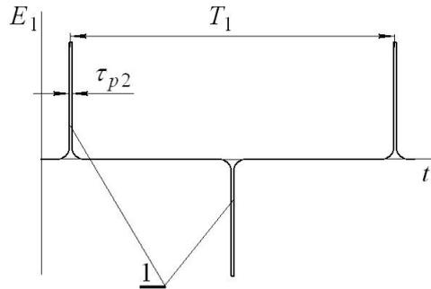
**Fig. 2** – Illustration of the concept of electromagnetic field femtosecond cluster. Here: 1 – clusters of electromagnetic field;  $E_1$  is the instantaneous electric field intensity of electromagnetic signal wave;  $T_1$  is the period of clusters;  $\tau_{p2}$  is the cluster duration;  $t$  is the time coordinate. Instantaneous picture is observed in the output plane of the electromagnetic cluster wave source
