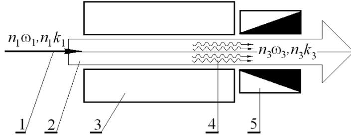
**Fig. 12** – Structural design of the resonance (parametric) modulator of the electron beam. Here: 1 – multiharmonic input signal (cluster signal wave with the frequency spectrum  $n_1\omega_1, n_1k_1$ ); 2 – nonmodulated electron beam; 3 – transverse undulator; 4 – modulated electron beam with the SCW packet (cluster SCW with the frequency spectrum  $n_3\omega_3, n_3k_3$ ); 5 – energy absorber of the cluster signal wave 1
