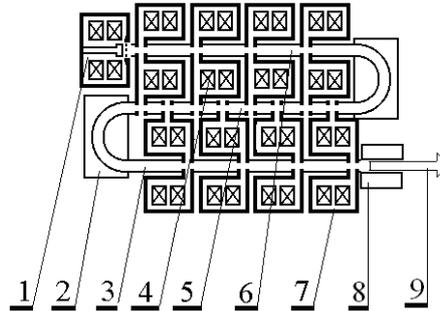
*Fig. 8 – Design diagram of the single-beam undulator induction electron accelerator with two internal and one external accelerating channels. Here: 1 – injector; 2 – turning systems; 3 – first internal accelerating channel; 4 – first linear accelerating unit; 5 – doubled external accelerating channel; 6 – second internal accelerating channel; 7 – second linear accelerating unit; 8 – output unit of the electron beam 9 formation*
