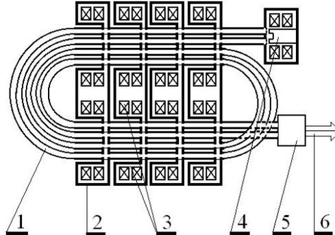
*Fig. 11* – Example of the structural design of two-beam induction accelerator-shaper of two-beam electron beam. Here: 1 – curvilinear channels in the turning systems (which for simplicity are not shown here); 2 – doubled eight-channel linear accelerating section; 3 – elliptic inductors of linear accelerating sections 2; 4 – two-beam injector; 5 – system of the double-speed beam formation
