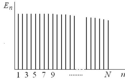
**Fig. 5** – Example of the spectrum of alternating periodic sequence of femtosecond clusters as “smear” Dirac delta functions. Here:  $E_n$  is the amplitude of the  $n$ -th harmonic of a signal;  $n$  is the sequential harmonic number;  $N$  is the upper number of the harmonic spectrum
