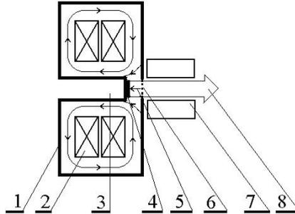
**Fig. 7** – Example of the design scheme of the single-beam induction electron injector. Here: 1 – electric screen; 2 – magnetic inductor; 3 – central electrode; 4 – cathode; 5 – force line of the internal part of the electric field, which is directly used for the beam 8 acceleration; 6 – transparent (for the beam 8) part of the electric screen 1 (anode, for example, is grid or foil); 7 – system of the electron beam 8 formation; 8 – output high-current electron beam
