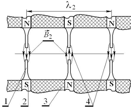
**Fig. 15** – Design of multiharmonic (cluster) magnetic undulator. Here: 1 – narrow magnetic tips; 2 – magnetic poles; 3 – magnetic insulator; 4 – force lines of the magnetic field of multiharmonic pump (magnetostatic clusters);  $\lambda_2$  is the undulation period (period of the first harmonic); N is the north magnetic pole; S is the south magnetic pole;  $\vec{B}_2$  is the vector of magnetic field induction
