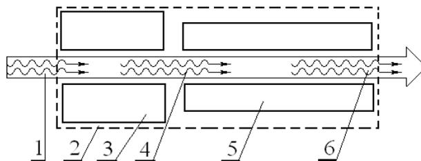
**Fig. 14** – Block diagram of the middle section in general case. Here: 1 – modulated electron beam coming from the modulator; 2 – middle section; 3 – active part of the middle section 2; 4 – multiharmonic modulated electron beam 2; 5 – passive part of the middle section 2; 6 – output multiharmonic modulated electron beam
