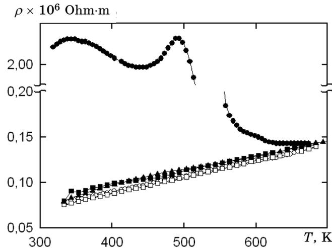
**Fig. 4** – Temperature dependence of the resistivity of Al film of the thickness  $d = 82$  nm: ●, ○ – I cycle; ■, □ – II cycle; ▲, △ – III cycle (dark – heating, light – cooling)
