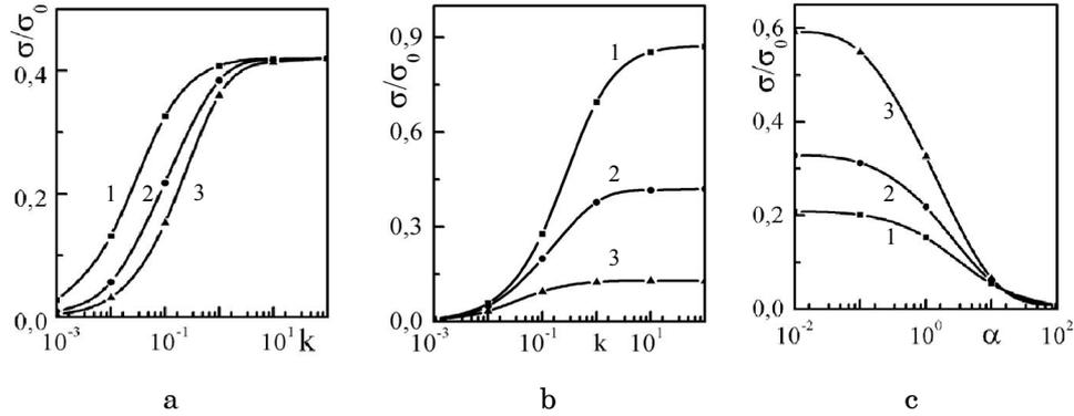
**Fig. 3** – Dependence of the conductivity of polycrystalline film on the normalized (to the electron free path) film thickness  $k$  (a, b) and the grain-boundary parameter  $\alpha$  at the following parameter values: a)  $\alpha = 1$ :  $1 - q_j = 0,8$ ,  $2 - q_j = 0,4$ ,  $3 - q_j = 0,0$ ; b)  $q_j = 0,1$ :  $1 - \alpha = 0,1$ ,  $2 - \alpha = 1$ ,  $3 - \alpha = 5$ ; c)  $k = 0,1$ :  $1 - q_j = 0,8$ ,  $2 - q_j = 0,4$ ,  $3 - q_j = 0,0$
