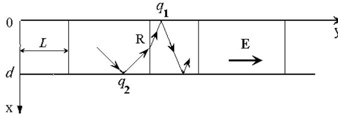
**Fig. 1** – Model of thin polycrystalline film where the possible motion path of a charge carrier is shown by the broken line:  $d$  is the film thickness;  $L$  is the average grain size in the sample surface;  $q_j$  ( $j = 1, 2$ ) is the probability of specular reflection of charge carriers by  $j$ -th outer boundary of the conductor;  $R$  is the probability of the diffusion scattering at the inter-grain boundaries;  $E$  is the electrostatic field strength
