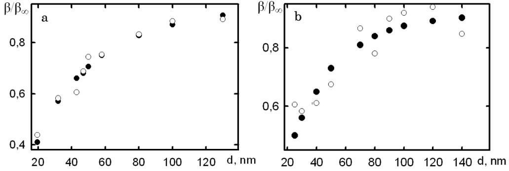
**Fig. 9** – Dependences of the temperature coefficient of resistance on the thickness for Al (a) and Ni (b) films:  $\circ$  – experiment,  $\bullet$  – calculation
