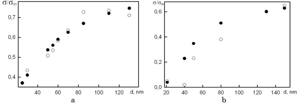
**Fig. 7** – Dependences of the conductivity on the thickness for Ni (a) and Al (b) films:  $\circ$  – experiment,  $\bullet$  – calculation
