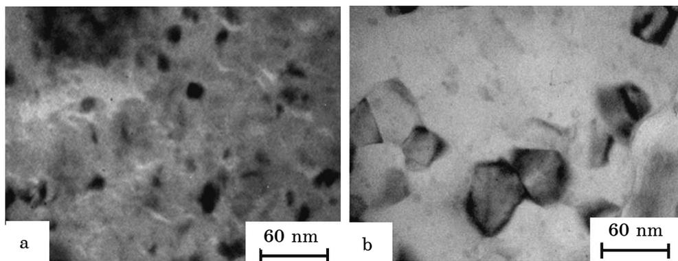
**Fig. 5** – Crystal structure of Ni (a) and Al (b) films of the thickness of 20 nm and 33 nm, respectively
