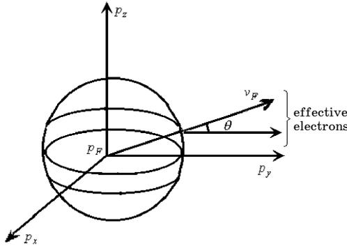
*Fig. 2 – For the calculation of the conductivity of thin film using the “inefficiency” conception of Pippard:  $p_\xi(\xi = x, y, z)$  are the components of quasi-impulse;  $v_F$  and  $p_F$  are the Fermi velocity and impulse, respectively*
