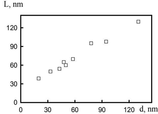
**Fig. 6** – Dependence of the average grain size on the Al film thickness. The annealing temperature is 700 K
