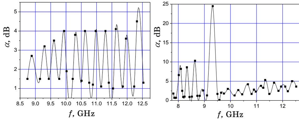
**Fig. 3** – Spectrum of the resonator with a metal screen on the lateral surface (a). Spectrum of the forced oscillations of the resonator with the grating at  $\theta = 0,3$  (b)
