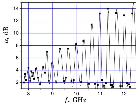
Fig. 2 – The spectrum of the resonator without screen
