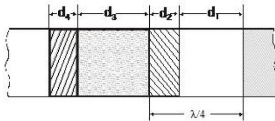
**Fig. 1** – Two-dimensional layered structure of the cell:  $d_1$  is the thickness of an empty waveguide adjacent to the short circuit;  $d_2$ ,  $d_4$  are the thicknesses of substrates confining the sample;  $d_3$  is the sample thickness
