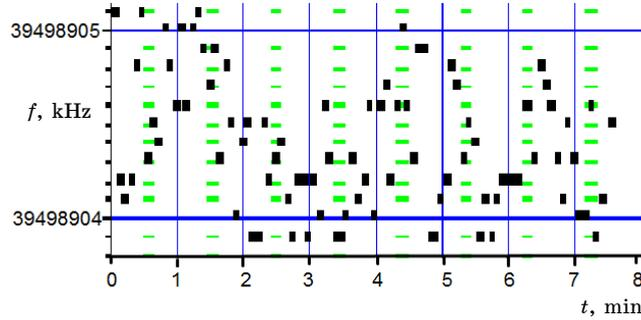
**Fig. 5** – Frequency deviation after temperature stabilization of the thermostat
