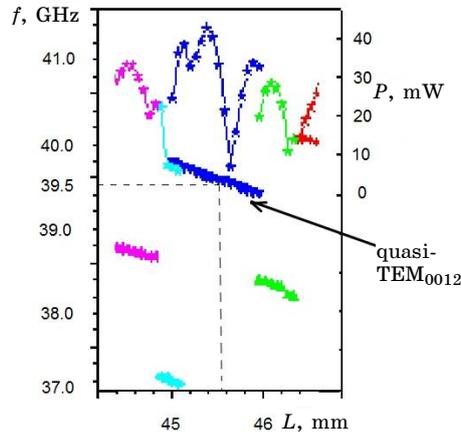
**Fig. 4** – Dependence of the frequency and the output power on the length of sphere-angle-echelette OR
