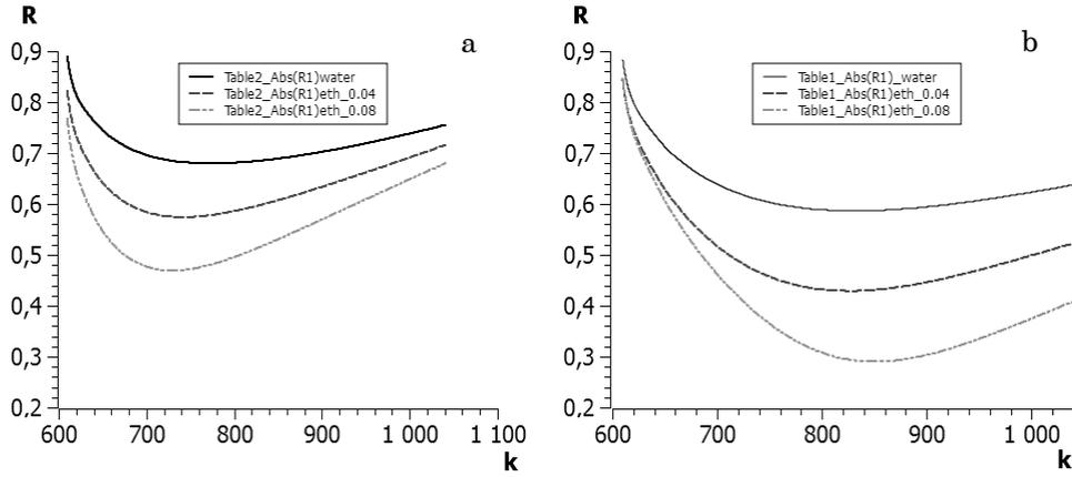
**Fig. 2** – Dependence of the modulus of the reflection coefficient ( $R$ ) of the simulated cell on the wave number ( $k$ ) at the thicknesses of the optimized substrate of 1,4 mm (a) and 0,8 mm (b) in the presence of the test substances in the structure
