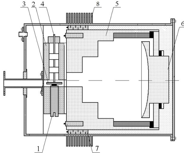
*Fig. 3 – Design of the quasi-optical solid-state oscillator*
