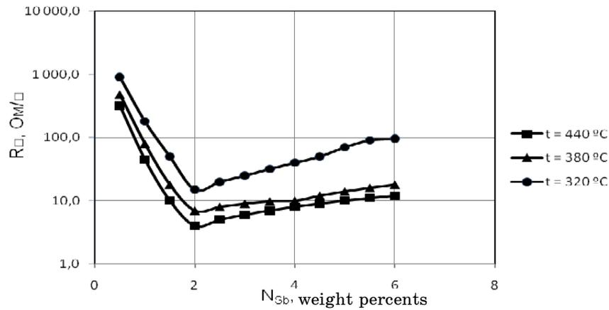
**Fig. 1** – Dependences of the surface resistance versus the antimony concentration at different deposition temperatures and  $\text{SnO}_2\text{:Sb}$  film thickness  $d = 500 \text{ nm}$
