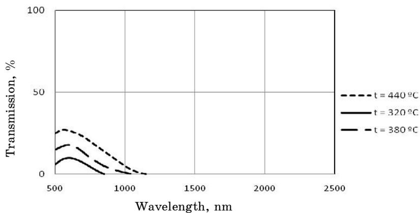
**Fig. 6** – Transmission spectrums of SnO<sub>2</sub>:Sb films, obtained with antimony concentration 1,8 weight percents at different temperatures
