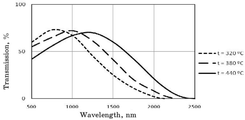
**Fig. 5** – Transmission spectrums of  $SnO_2:Sb$  films, obtained with antimony concentration 0,5 weight percents at different temperatures
