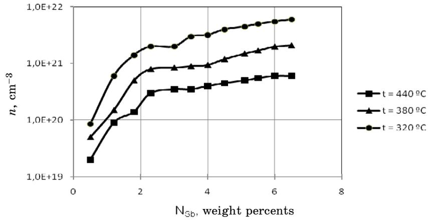
**Fig. 4** – Dependences of the charge carrier concentration versus the antimony concentration at different deposition temperatures and  $SnO_2:Sb$  film thickness  $d = 500$  nm
