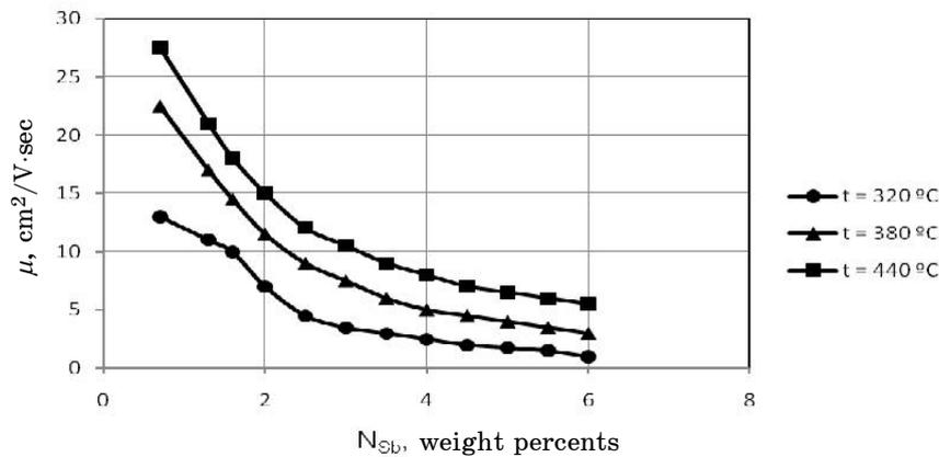
**Fig. 3** – Dependences of the charge carrier mobility versus the antimony concentration at different deposition temperatures and SnO<sub>2</sub>:Sb film thickness  $d = 500$  nm
