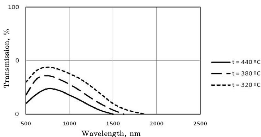
**Fig. 7** – Transmission spectrums of SnO<sub>2</sub>:Sb films, obtained with antimony concentration 3,5 weight percents at different temperatures
