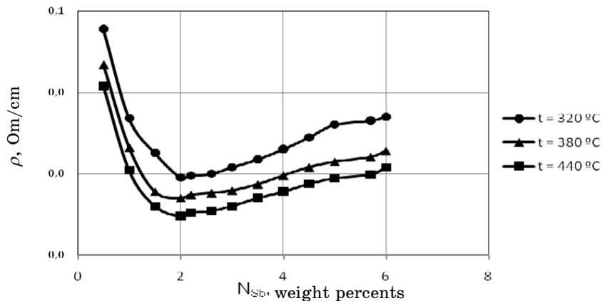
**Fig. 2** – Dependences of the resistivity versus the antimony concentration at different deposition temperatures and  $\text{SnO}_2\text{:Sb}$  film thickness  $d = 500 \text{ nm}$
