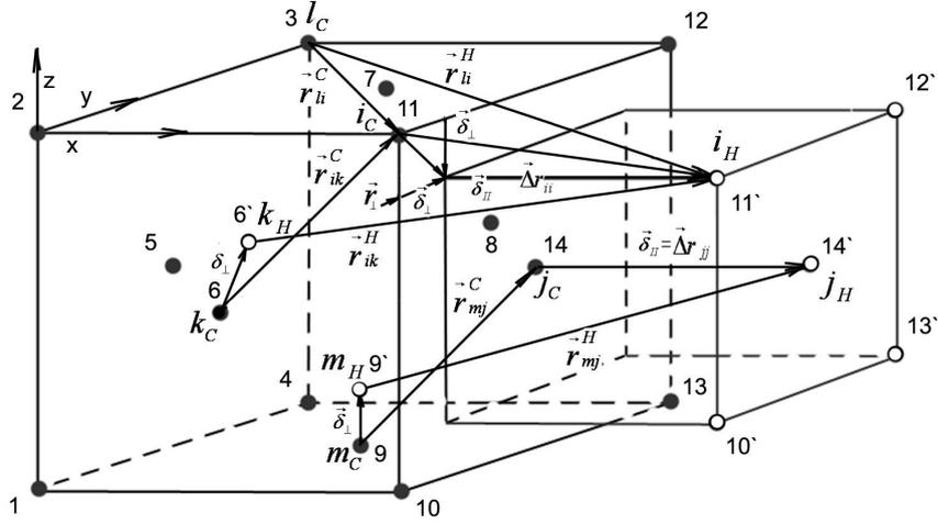
Fig. 1 – Diagram of the forces, acting in the sections of deformed cell
