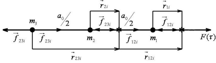
**Fig. 3** – Forces action on the reduced masses in an arbitrary time moment under the external force  $\vec{F}(\tau)$  influence. Dots denote the initial positions of reduced masses in a cell; asterisks present the positions of reduced masses in a cell in an arbitrary time moment
