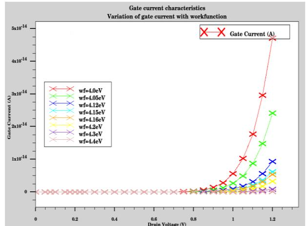
Fig. 5 –  $I_G$  versus  $V_D$  Plot for different values of gate work-functions
