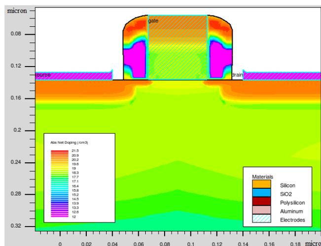
Fig. 1 – Structure of lightly doped 45 nm NMOS
