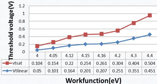
Fig. 6 – Variation of threshold voltage at higher drain voltage with work-function
