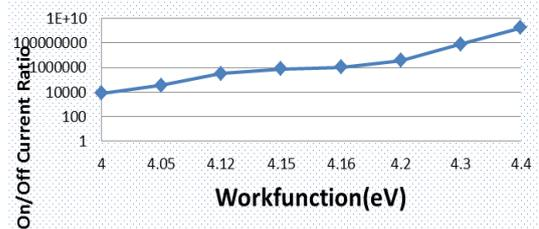
Fig. 8 – Variation of On/Off current with work-function
