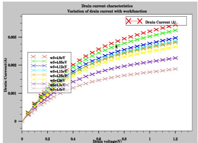
Fig. 4 –  $I_D$  versus  $V_D$  Plot for different values of gate work-functions
