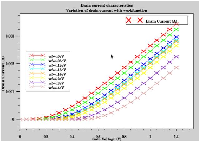
Fig. 2 –  $I_D$  versus  $V_G$  Plot in linear Scale for different values of gate work-functions
