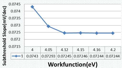
Fig. 9 – Variation of SSlinear with work-function
