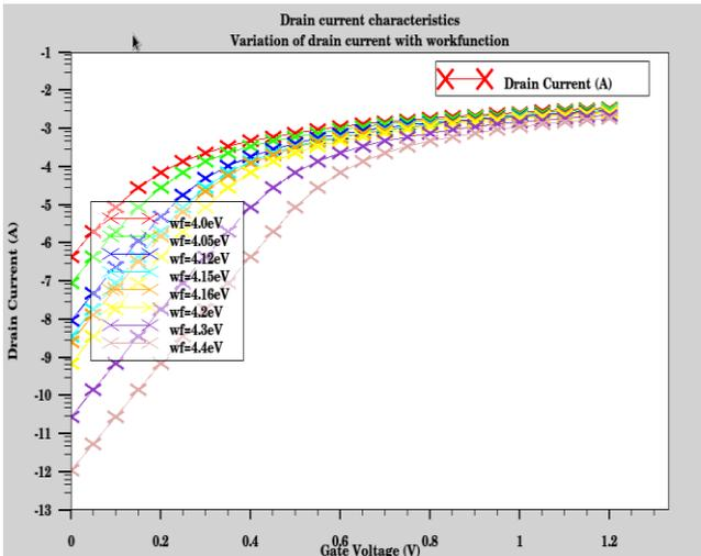
Fig. 3 –  $I_D$  versus  $V_G$  Plot in Log Scale for different values of gate work-functions
