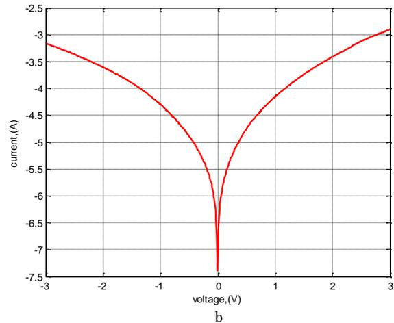
**Fig. 4** – Experimental current-voltage characterization of Au-GaAs Schottky diode (a) in a linear (b) and a semi-logarithmic illustration
