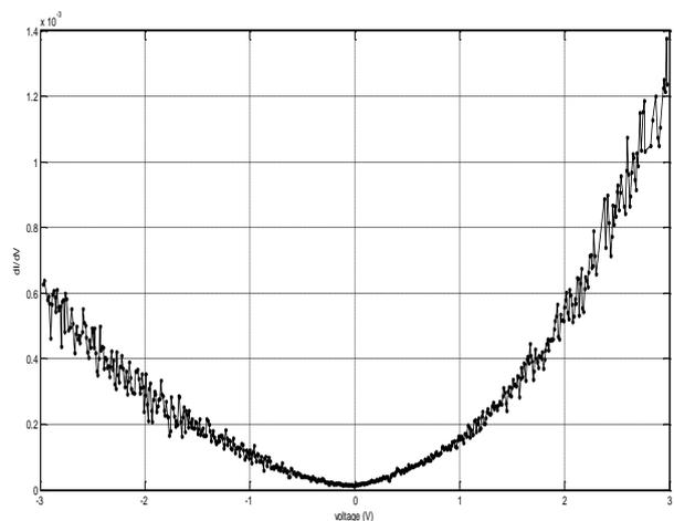
**Fig. 6** – SBD conductivity versus DC Bias of Au-GaAs
