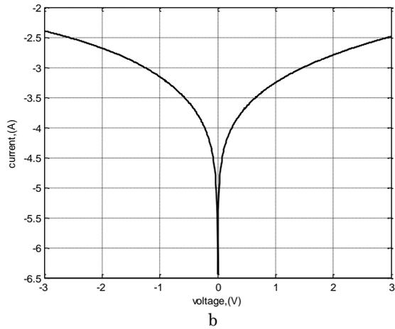
**Fig. 3** – Experimental current-voltage characterization of Au-InP Schottky diode (a) in a linear (b) and a semi-logarithmic illustration
