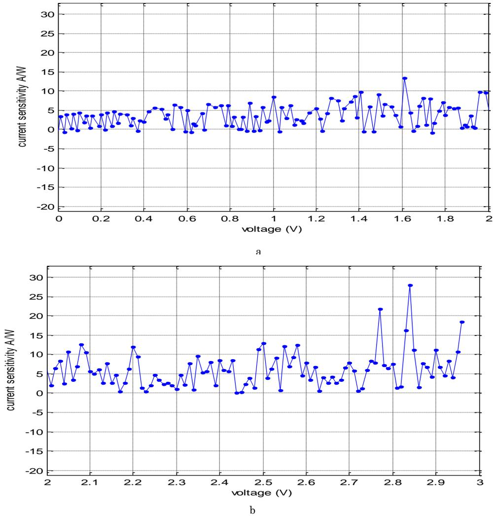
**Fig. 7** – SBD sensitivity versus DC Bias of Au-InP (a) Low values of forward bias, (b) High values of forward bias
