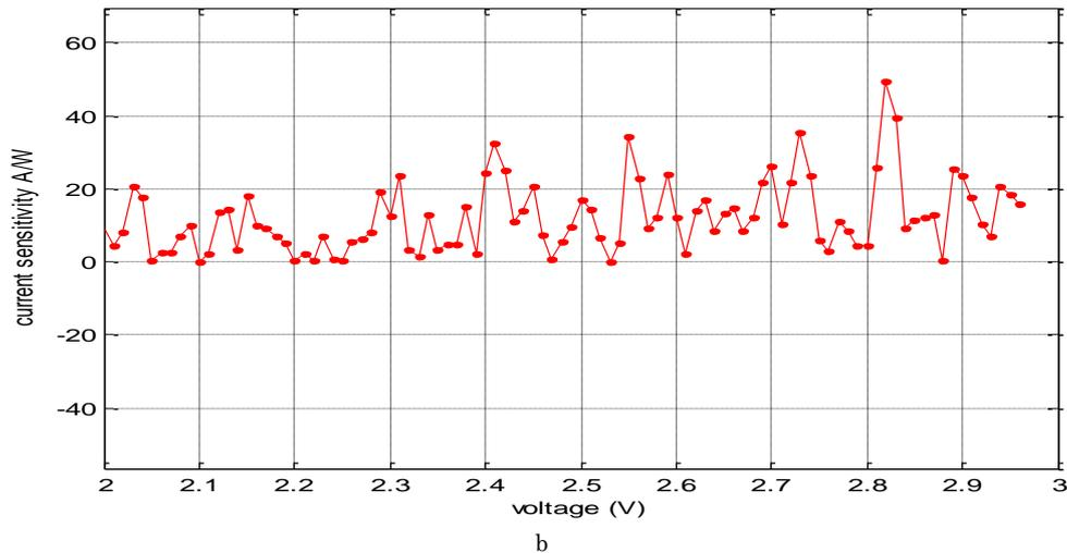
Fig. 8 – SBD sensitivity versus DC Bias of Au-GaAs. (a) Low values of forward bias, (b) High values of forward bias
