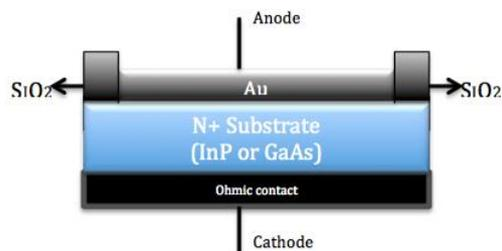
Fig. 1 – Structure of Schottky barrier diode detector
