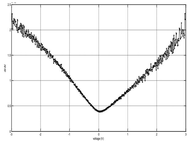
**Fig. 5** – SBD conductivity versus DC Bias of Au-InP
