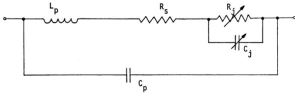
Fig. 2 – Equivalent Circuit for SBD
