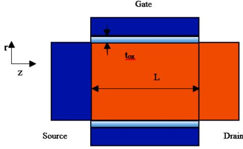
Fig. 1 – A GaSb-InAs Heterojunction Gate All Around TFET
