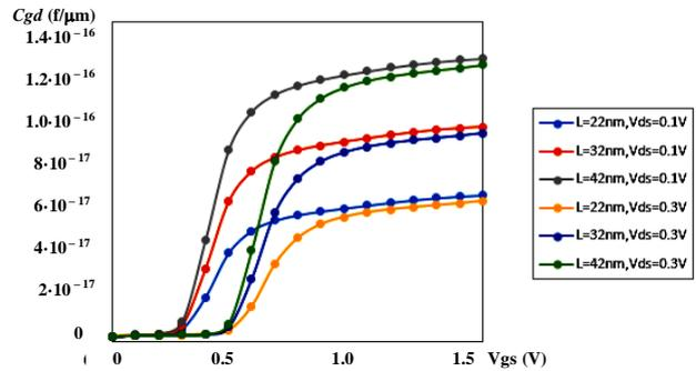
Fig. 5 – Gate-drain capacitance at  $L_g = 22$  nm, 32 nm, 42 nm with  $N_d = 10^{18}/\text{cm}^3$
