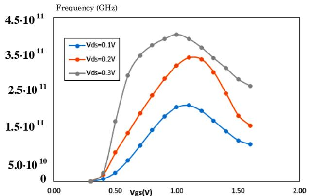
Fig. 6 – Cut-off frequency at  $L_g = 22$  nm,  $N_d = 10^{18}/\text{cm}^3$
