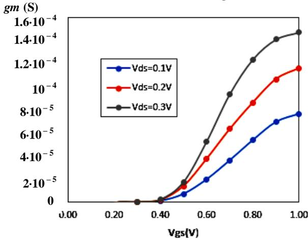
Fig. 3 – Transconductance at  $L_g = 22$  nm,  $N_d = 10^{18}/\text{cm}^3$
