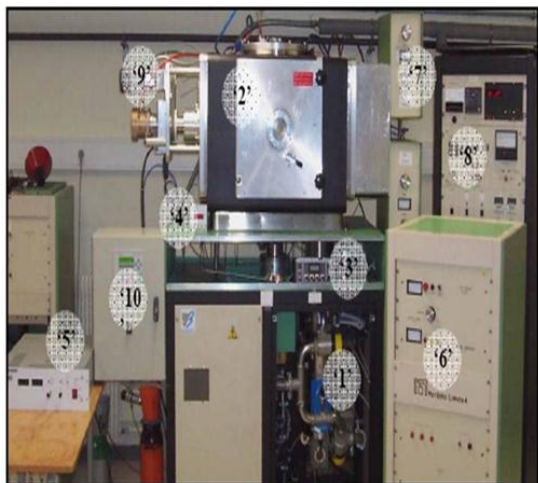
Fig. 1 – Magnetron sputtering system. '1' pumping system, '2' filing cabinet, '3' mass flowmeters, '4' pressure drive, '5' DC power supply, '6' 13.56 MHz RF generator, '7' stub, '8' quadrant control, '9' turntable motor substrate holder (PS), '10' automaton
