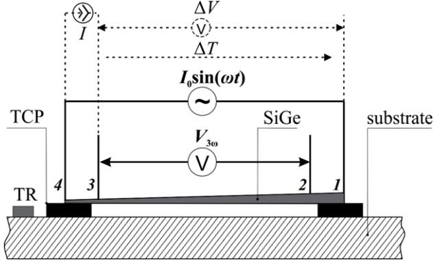
**Fig. 1.** – Schematic view of the setting for thermal conductivity measurements by  $3\omega$ -method (solid lines) and for measurements of Seebeck coefficient (dashed lines) of SiGe whiskers. In the latter case, the part of whisker is heated by current  $I$ , which is passed between two adjacent electrodes (here, 3 and 4), and the thermo-e.m.f.  $\Delta V$  induced due to temperature difference  $\Delta T$  is measured between the hot and cold ends (here, 3 and 1, respectively)
