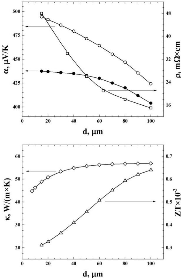
**Fig. 4.** – Changes of Seebeck coefficient  $\alpha$  and resistivity  $\rho$  (top) and of thermal conductivity  $\kappa$  and  $ZT$  (bottom) with effective diameter of oblique  $\text{Si}_{0.97}\text{Ge}_{0.03}$  ( $N_A = 3 \times 10^{18} \text{ cm}^{-3}$ ) at 300 K. Diameter dependence of thermal conductivity has been estimated basing on the data from [15]. Solid circles represent the diameter dependence of Seebeck coefficient for straight (non-oblique) whiskers
