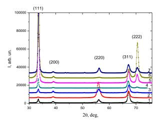
**Fig. 3** – Plots X-ray diffraction spectra of coatings ZrN, obtained by  $P_{\rm N}=0.65$  Pa,  $U_{ip}=-1200$  V and  $U_b$ : 1-27 V; 2-40 V; 3-70 V; 4-100 V; 5-150 V; 6-220 V; 7-300 V
