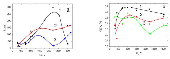
Fig. 6 – The dependence of the crystallite size (a) and microstrain (b) from the constant potential at  $P_N = 0.65$  Pa:  $1 - U_{ip} = 0$  V;  $2 - U_{ip} = -1200$  V;  $3 - U_{ip} = -2000$  V
