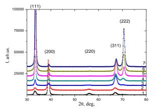
**Fig. 2** – Plots X-ray diffraction spectra of coatings ZrN, obtained by  $P_{\rm N}=0.65$  Pa,  $U_{ip}=0$  V,  $U_{b}$ : 1 – 27 V; 2 – 40 V; 3 – 70 V; 4 – 100 V; 5 – 150 V; 6 – 220 V; 7 – 300 V
