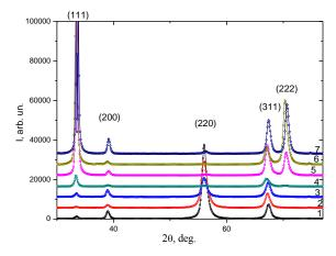
**Fig. 4** – Plots X-ray diffraction spectra of coatings ZrN, obtained by  $P_{\rm N}=0.65$  Pa,  $U_{ip}=-2000$  V and  $U_b$ : 1--27 V; 2--40 V; 3-70 V; 4-100 V; 5-150 V; 6-220 V; 7-300 V
