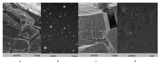
Fig. 1 – The surface morphology and fractographs breaks ZrN coatings ( $P_N = 0.65 \text{ Pa}$ ): a, b –  $U_b = -40 \text{ V}$ ; c, d –  $U_b = -220 \text{ V}$
