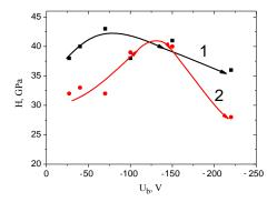
Fig. 7 – Dependence of the microhardness of coatings from values of the constant potential at  $P_{\rm N}=0.65$  Pa:  $1-U_{ip}=0$  V,  $2-U_{ip}=-2000$  V
