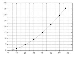
Fig. 3 - The depth of penetration of beta particles in Si
