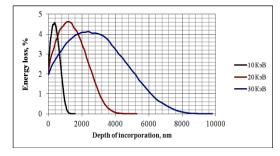
Fig. 4 – Dependence of the energy losses of electrons
