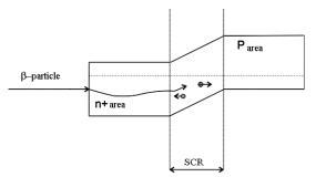
Fig. 1 - Principle of betavoltaic battery work
