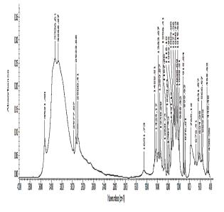
Fig. 3 – IR spectrum of lactobionic acid
