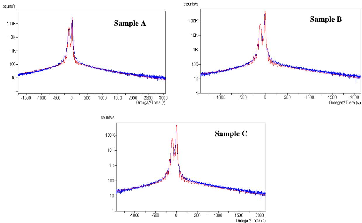
**Fig. 4** – HRXRD rocking curve (a) Sample A (b) Sample B (c) Sample C; Blue shows the experimental measurement data and red line shows the simulation
