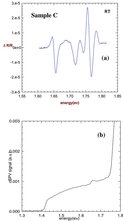
Fig. 3 – RT (a) PR (b) SPS spectra of sample C
