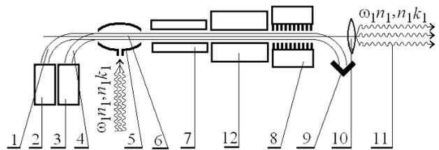
**Fig. 4** – Structural scheme of two-stream cluster FEL-klystron with non-resonant modulator 7 and system of intermediate acceleration of an electron beam 12
