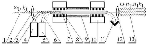
**Fig. 1** – Structural scheme of two-stream cluster FEL-klystron with resonant modulator 8 and monochromatic input signal 1
