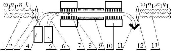
**Fig. 2** – Structural scheme of two-stream cluster FEL-klystron with resonant modulator 8 and multiharmonic input signal 1
