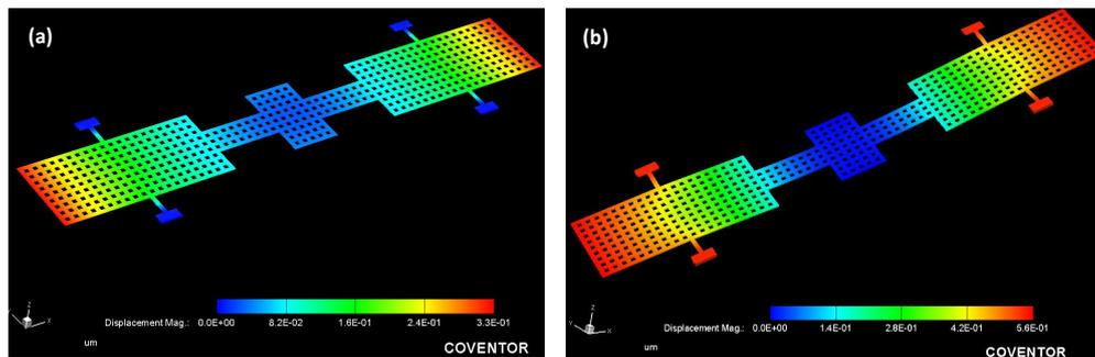
**Fig. 4** – (a) Simulated response of STS with multilayer movable membrane composed of Cr-Au-Au-Ti-Au, at room temperature, showing a maximum deflection of 0.33  $\mu\text{m}$ , (b) Simulated response of STS with multilayer movable membrane composed of Cr-Au-Au-Ti-Au, at 70 °C, showing a maximum deflection of 0.56  $\mu\text{m}$
